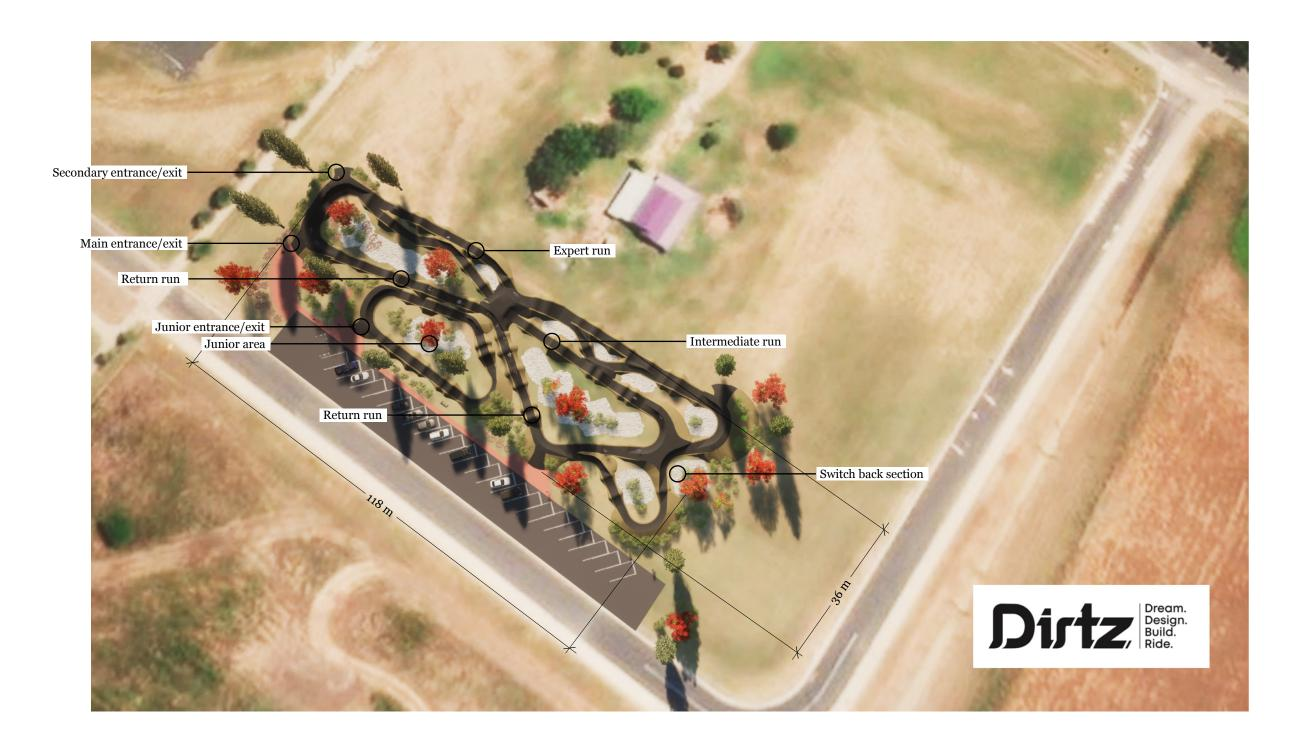
The Pump/Jump park is separated into separate runs.:
