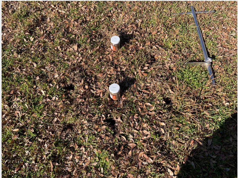
Sample site 12 cores in 500 mm x 600 mm grid
