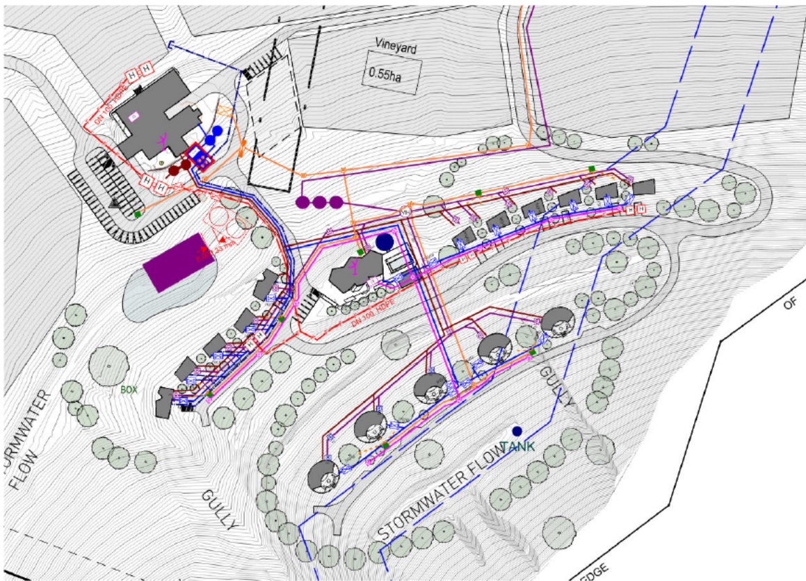
Image 1: Image showing 1 way alternative access to public road and proposed hydrant locations.
