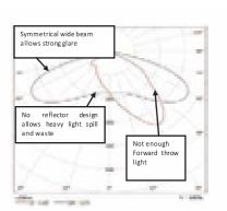
Specific photometric increases the uniformity of light, while reducing the light spill outside the court.
