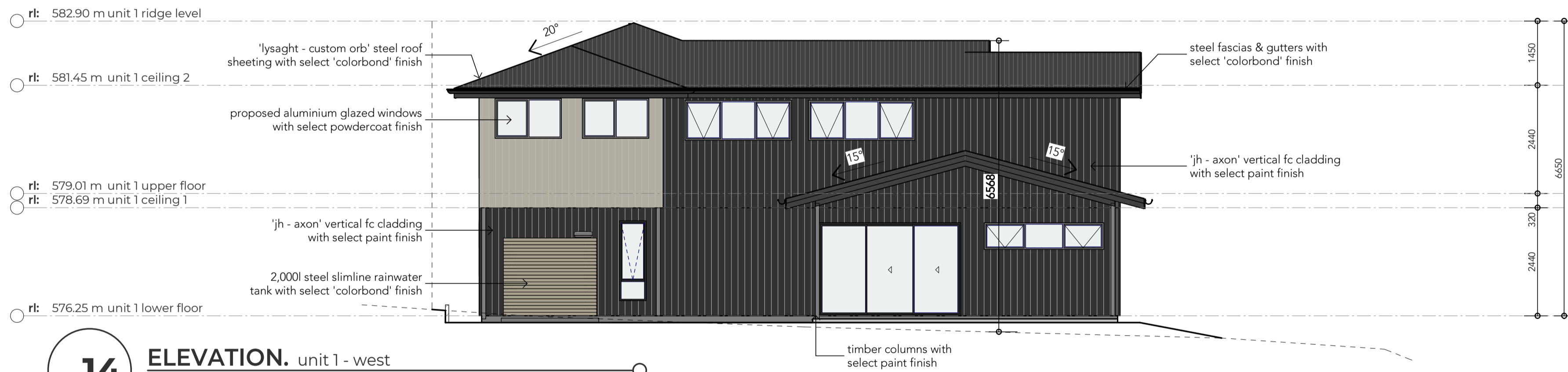
14 ELEVATION. unit 1 - west
