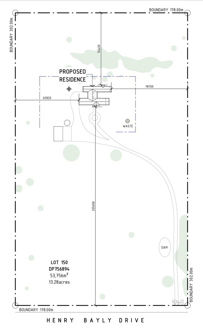
02 SCALE: 1 : 1200 (A3) 0 12000 24000 48000 96000 LEGEND: DENOTES BUILDERS ALLOCATED WASTE AREA DURING CONSTRUCTION - DENOTES SEDIMENT CONTROL BARRIER 2,40 DENOTES TEMPORARY GRAVEL CONSTRUCTION EXIT
