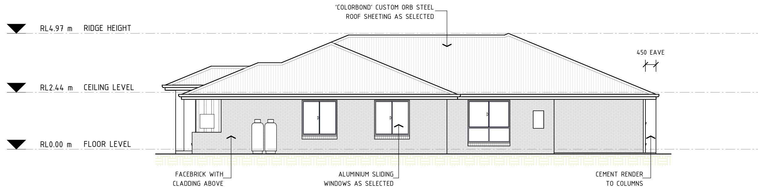
07 | ELEVATION: EAST FACADE SCALE: 1 : 100 (A3)
