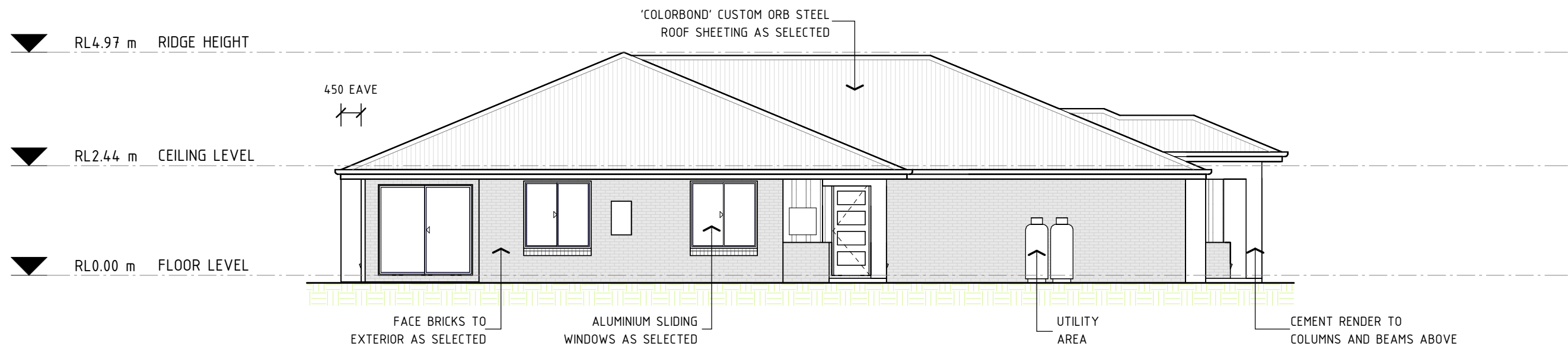
05 | ELEVATION: WEST FACADE SCALE: 1 : 100 (A3)
