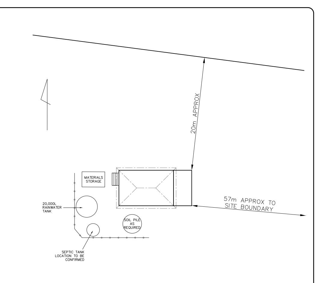
\* ALL DIMENSIONS ARE TO BE CONFIRMED BY THE BUILDER PRIOR TO CONSTRUCTION. DO NOT SCALE FROM DRAWINGS. BUILDING SET OUT & SITE BOUNDARY DETAILS TO BE CONFIRMED BY A REGISTERED SURVEYOR. ALL WORK TO BE CARRIED OUT TO RELEVANT STANDARDS AND BUILDING CODES.
