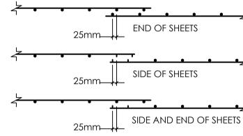
C26 A 0.2mm POLYETHYLENE MEMBRANE SHALL BE CONTINUOUS UNDER SLAB LAPPED 200mm MIN. WHERE REQUIRED AND TAPED AT ALL SERVICE PENETRATIONS, LAPS AND PUNCTURES THE MEMBRANE IS TO EXTEND UNDER AND TO THE SIDES OF SLABS, BEAMS AND THICKENINGS.
