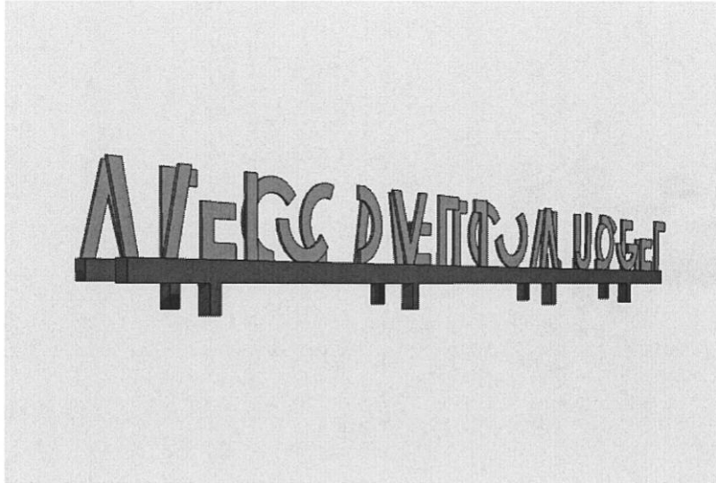
Slide 1 Welcome to Mudgee sign. 10mm laser cut rusting steel on black steel base.
