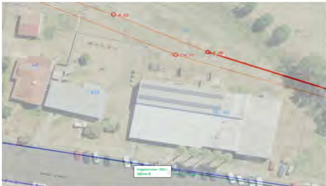
Figure 2.3 – Irrigation main - 300mm pipework location shown in green
