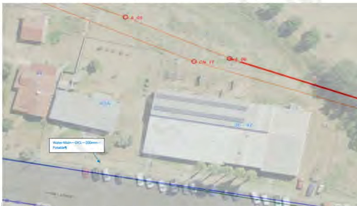
Figure 2.1 – Water main - 200mm pipework location shown in blue
