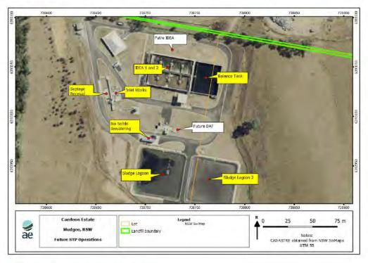
Figure 6: STP Odour Sources (Current)
