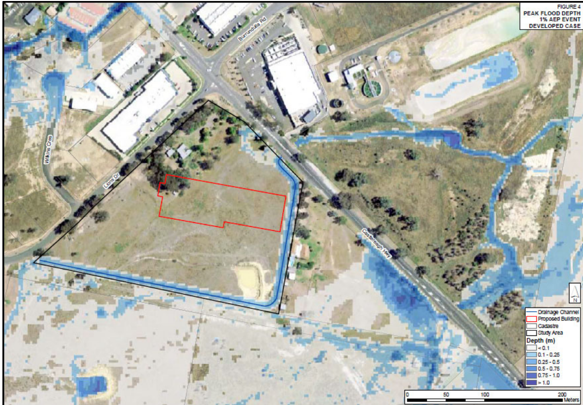
Figure 7: Extract from WM Water Flood Assessment showing modelling of peak flood depth in 1%AEP event post development
