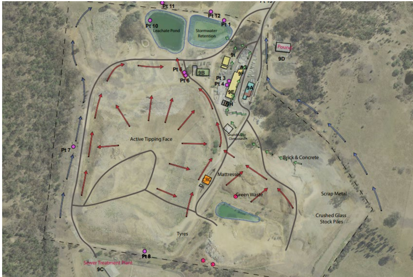
Figure 2 – Stormwater drainage of the Mudgee Waste Facility
