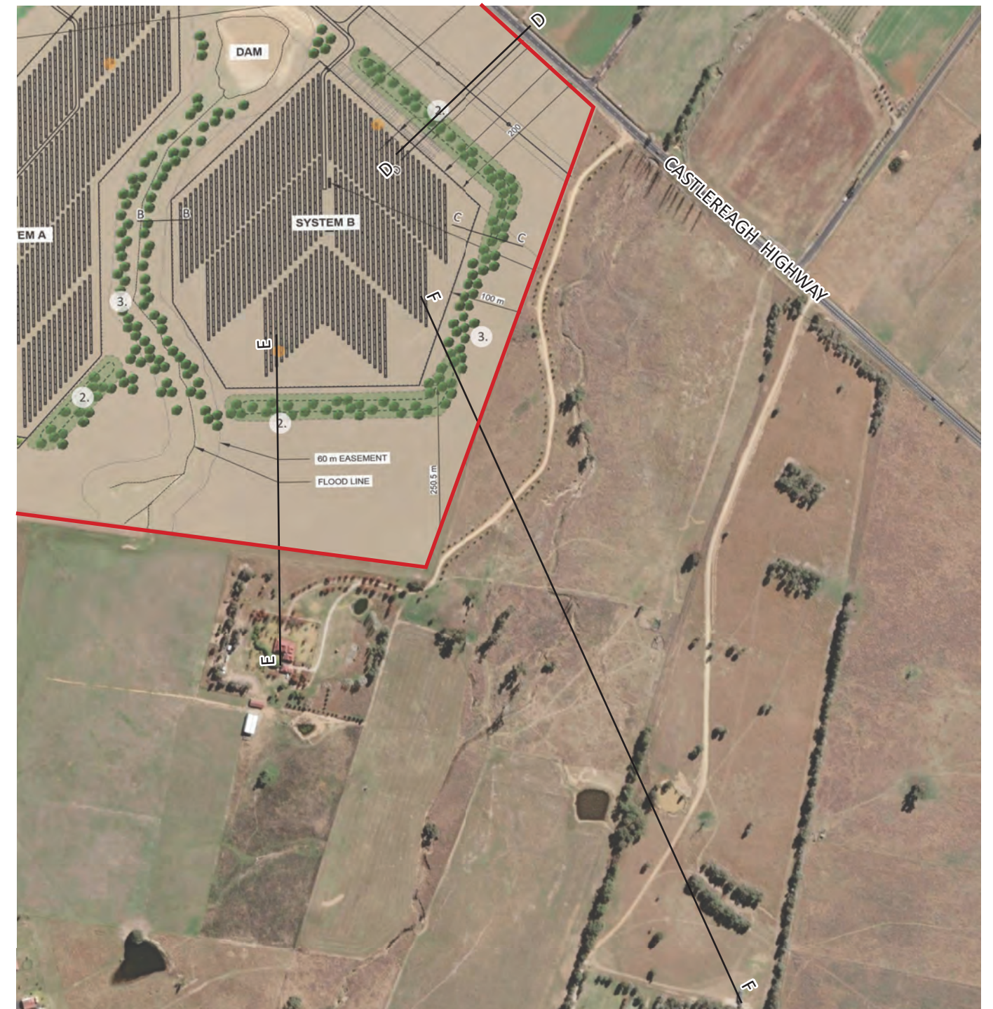
E - E Long section showing screening effect of mounding on view from dwelling at 312 Castlereagh Highway
