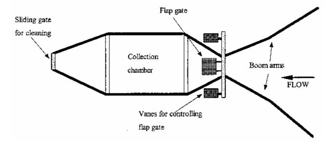
Figure 1.8 Schematical layout of Bandalong Boom
