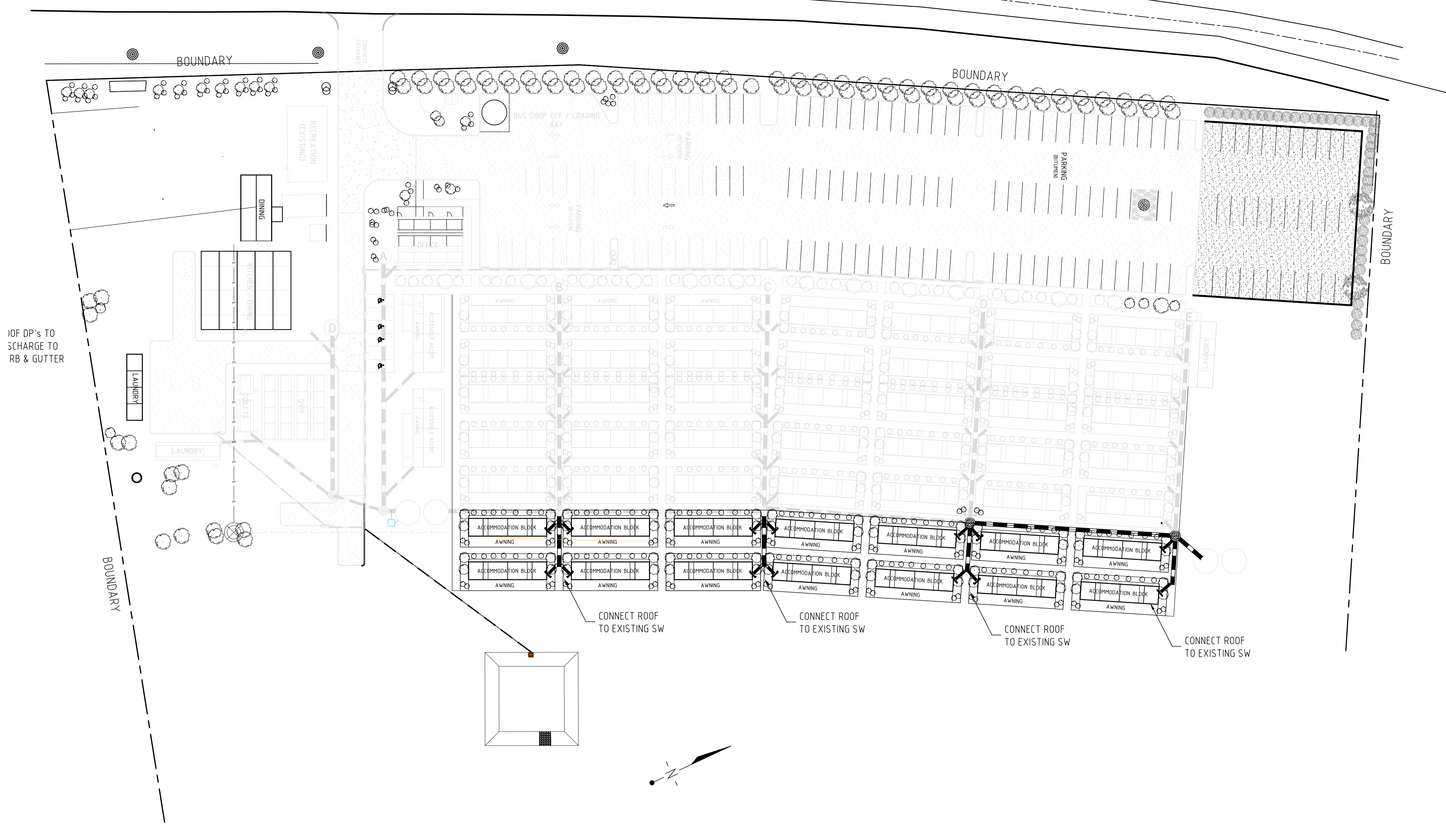
GENERAL ARRANGEMENT ROOF STORMWATER MANAGEMENT PLAN SCALE = 1:400
