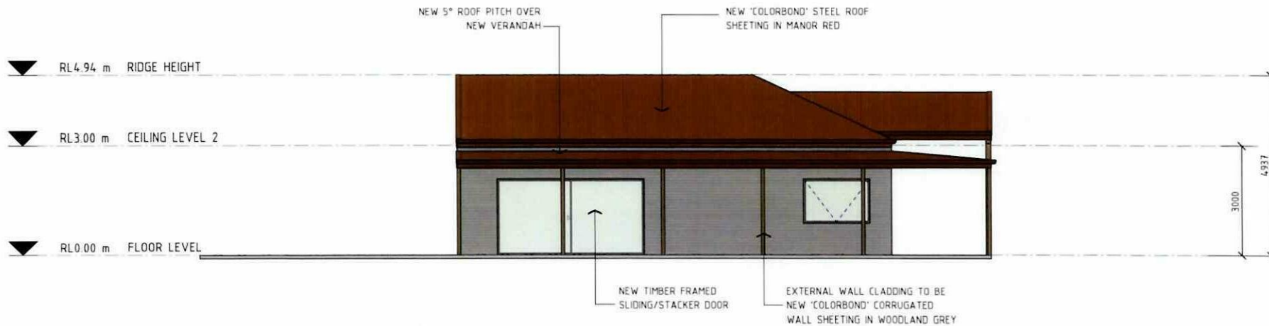
04 ELEVATION: SOUTH FACADE SCALE: 1:100 (A3)
