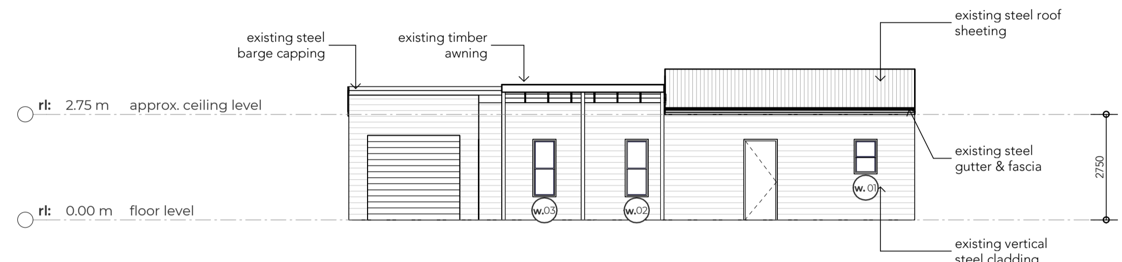
04 ELEVATION. EAST FACADE Scale 1 : 100 @ A1
