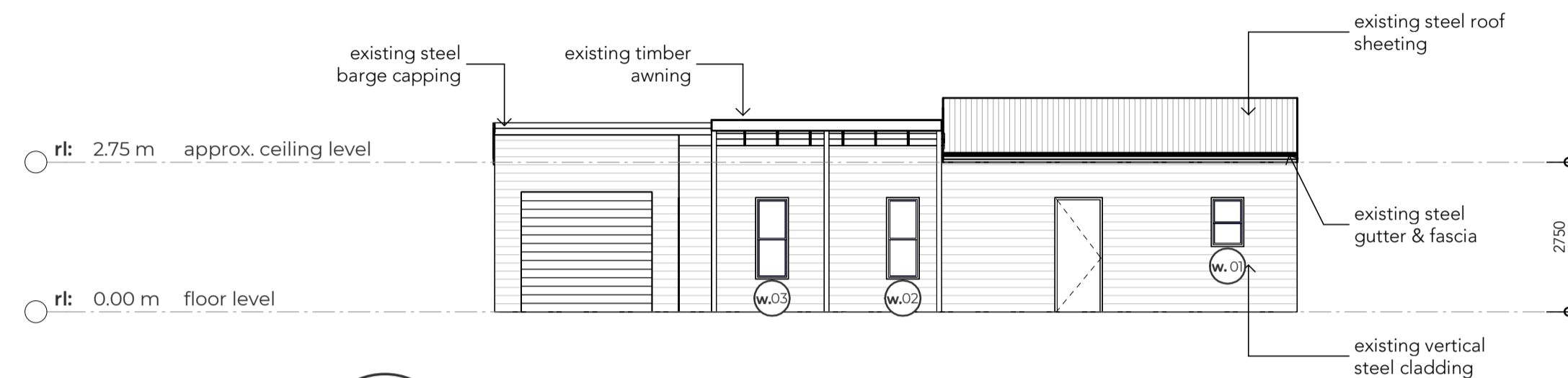
04 ELEVATION. EAST FACADE Scale 1 : 100 @ A1
