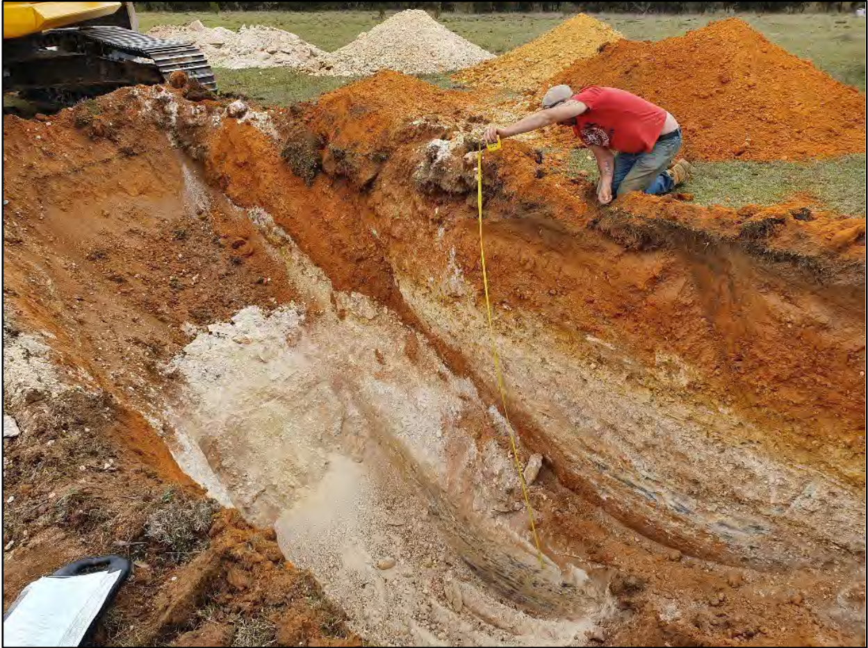
Plate 8: Typical Soil Profile Onsite
