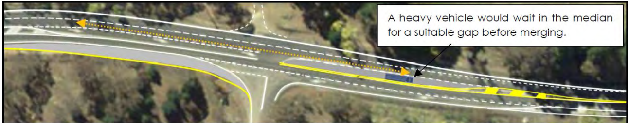
Figure 12: Typical Acceleration Lane Extension
