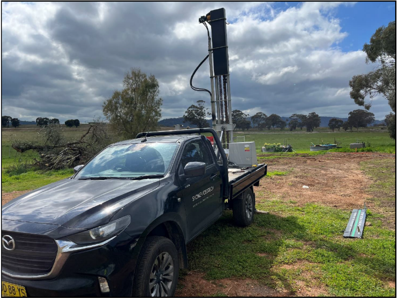
Figure 1 4WD Ute Mounted Drilling Rig
