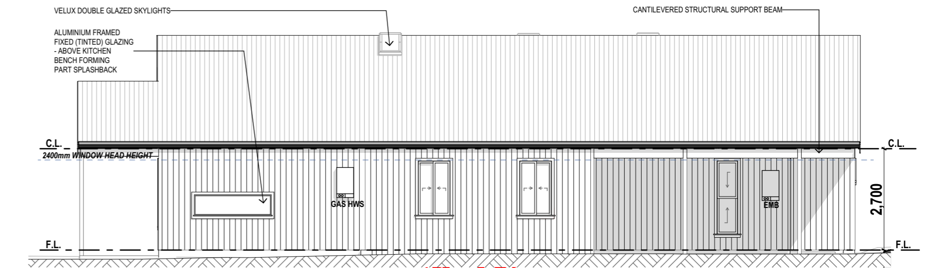
E-09 WEST ELEVATION - UNIT 2 1:100
