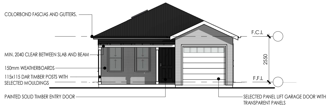
1 SOUTH ELEVATION SCALE 1 : 100
