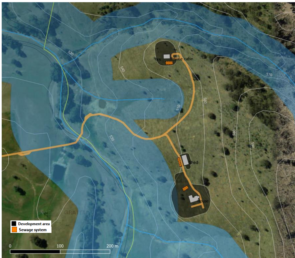
Figure 5-1. Proposed site layout and location of sewage systems in relation to the 100m buffer to Macdonalds Creek and 40 buffer from side tributaries.
