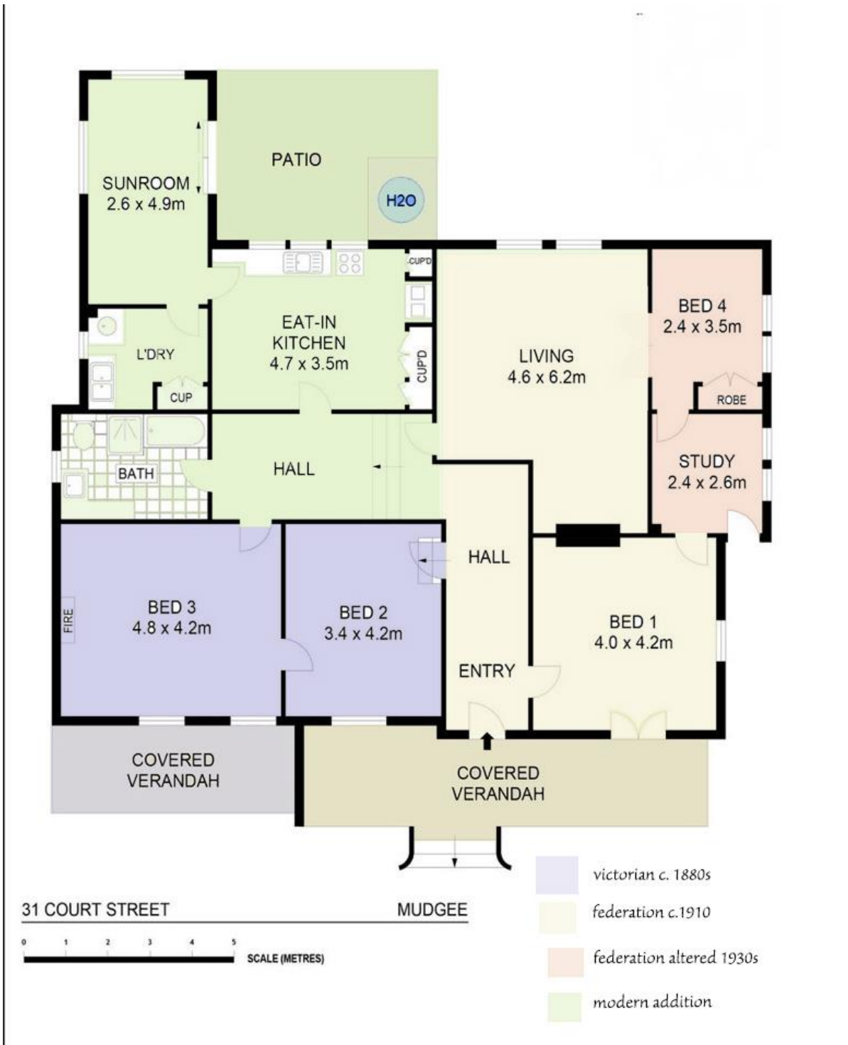
Figure 8 Periods of construction at 31 Court Street.
