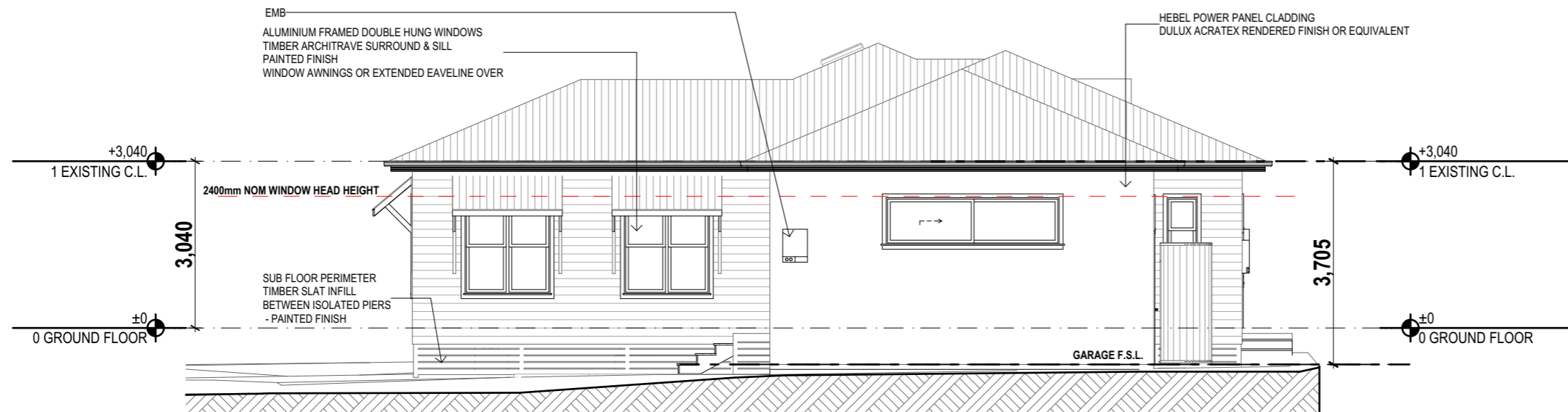
E-01 WEST ELEVATION 1:100
