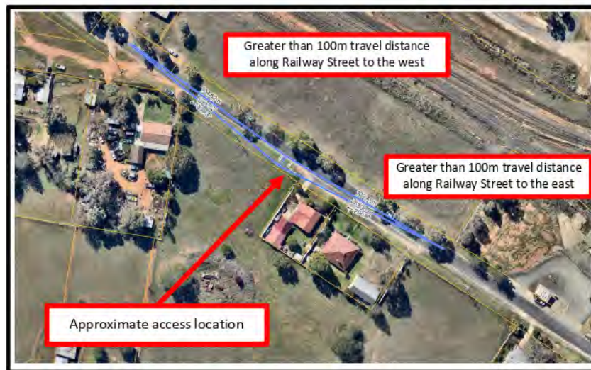
FIGURE 10 SIGHT DISTANCE REVIEW OF THE PROPOSED ACCESS JUNCTION
