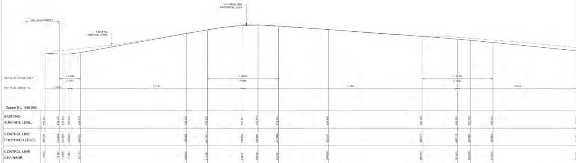
ROAD 1 - LONGITUDINAL SECTION SCALE (H) 1:500 (V) 1:100
